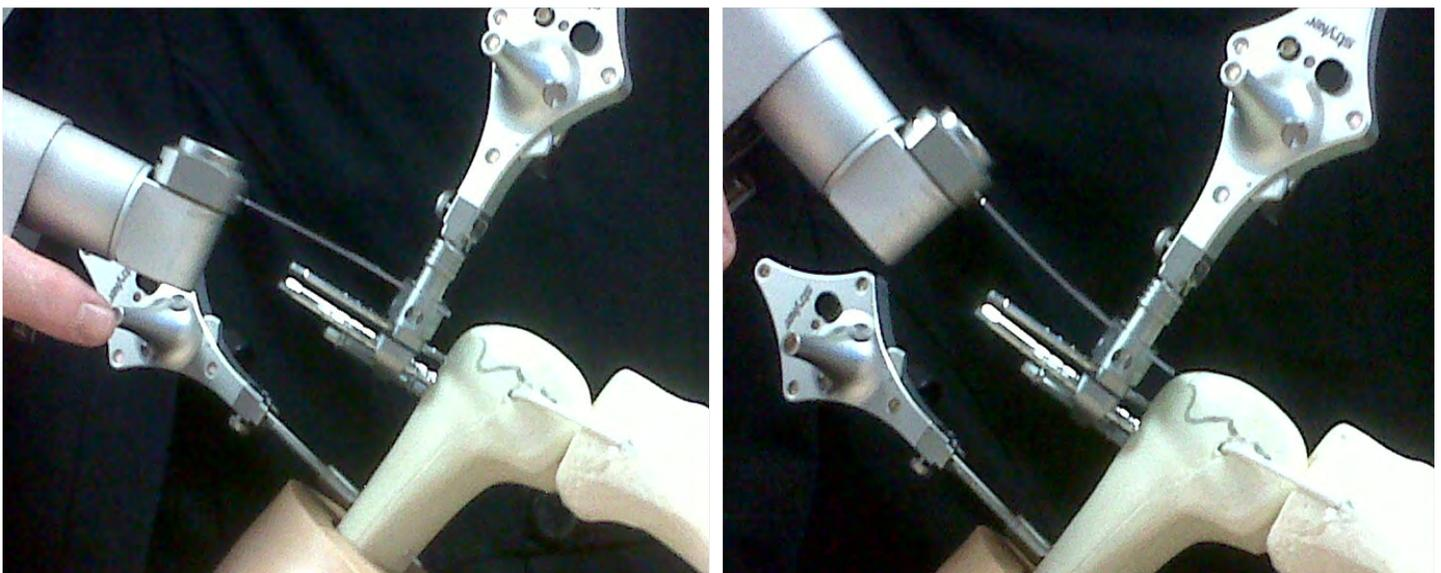
**Figure 2.** Bending of the saw blade by either 'hanging' the saw (left image) or 'lifting' the saw (right image).
